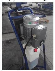
Step3, Connect fitting and oilhose from engine to piston.
